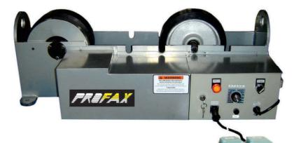
Maximum load capacity 5,000 lbs. (set) (2,500 lbs. max for each the drive and idler) \*Maximum rotational capacity 7,500 lbs. with additional idlers.
